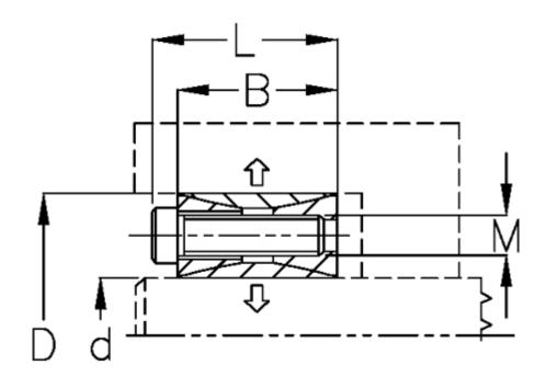
$\begin{array}{lll} \text{B mm} & = 28 \\ \text{d H8 mm} & = 80 \\ \text{D mm} & = 120 \\ \text{Fit tolerance} & = \text{Aksel k11-h11, Nav N11-H11} \\ \text{F kN torque} & = 83.6 \\ \text{L mm} & = 38 \\ \text{M mm} & = \text{M10} \\ \text{P N/mm2 surface pressure on shaft/hub} = 47 \end{array}$
